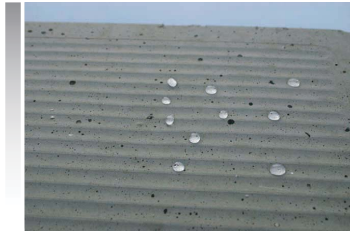
Concrete part 24 hours after pouring. Water droplets will not absorb Below : same sample after breaking . Water on the break zone
