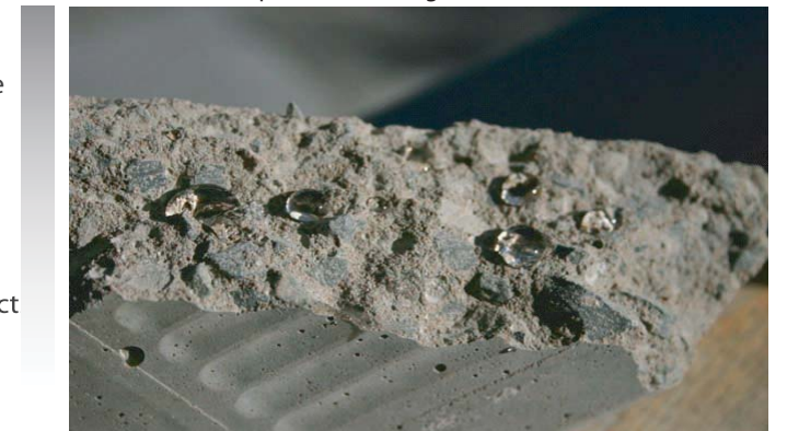
Concrete part 24 hours after pouring. Water droplets will not absorb Below : same sample after breaking . Water on the break zone
