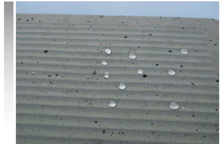
Concrete part 24 hours after pouring. Water droplets will not absorb Below : same sample after breaking . Water on the break zone
