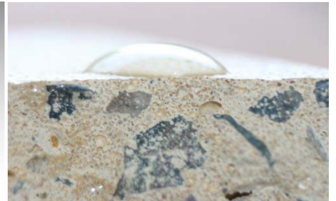
Absorption comparison 16 month after the application Single pavers treated.
