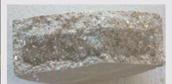
After the curing and stored in water for 24 hours. Significant reduced water absorption as deep as 3001 penetrates.
