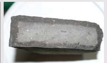
Deep penetration. This sample was split in half, 2 hours after the surface application of 200 ml /m2 3001
